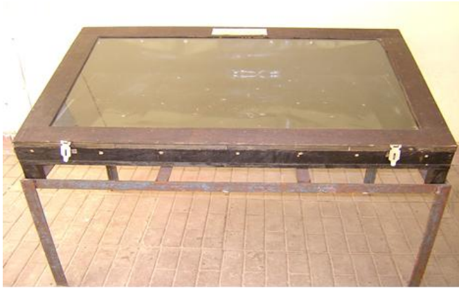
Figure 1. Natural convection type solar dryer.
