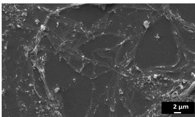
**Fig. 4 MLG film transferred to a Si wafer.**
